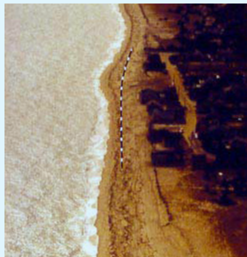
Figure 15: STABEACH dewatering system in Cod Fish Park, Nantucket. Dashed line indicates the location of the buried dewatering pipe. Note the bulge in the shoreline generated by the deposition of sediment in the swash zone over the pipe (Photograph courtesy of Coastal Stabilization, Inc.).
